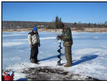
Drilling through the 60-cm-thick ice at the surface of Bark Bay Slough. Photo by M. Du.
