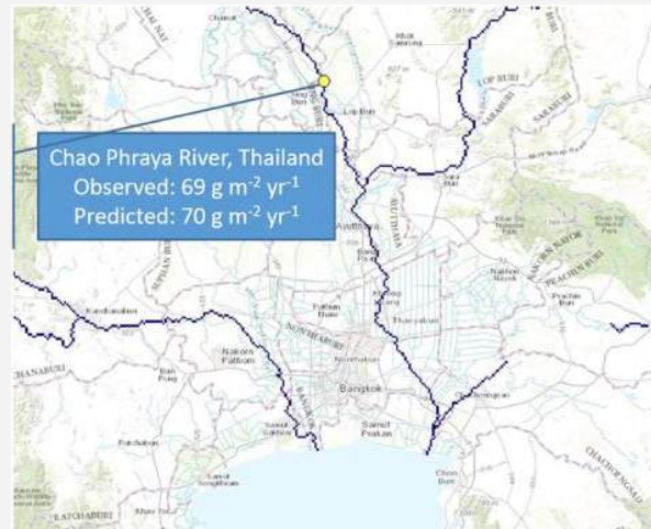
An example output of the sediment flux model, showing the Chao Phraya River in Thailand. This is an example of one of the best model predictions relative to observed data. The model predicts the annual sediment yield for every 30 arc-second grid cell across the globe.
