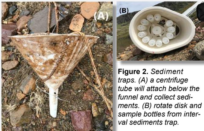
**Figure 2.** Sediment traps. (A) a centrifuge tube will attach below the funnel and collect sediments. (B) rotate disk and sample bottles from interval sediments trap.
